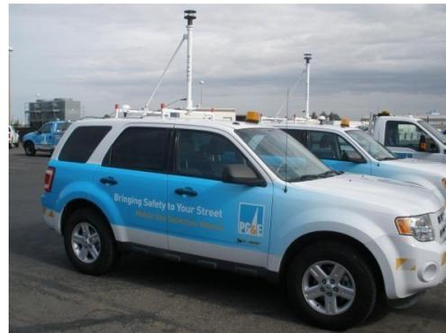
Above: PG&E fleet vehicle with top-mounted leak sensor
